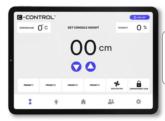
Cooling Fan - Controls the switching on and off of the cooling fans inside the CPU cabinet for heat and ventilation control.
